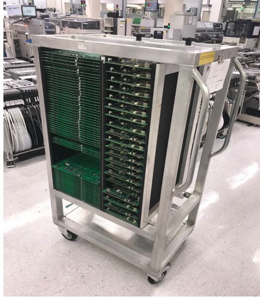
Figure 4.1: Transport Trolley: Batch Transport Mechanism
