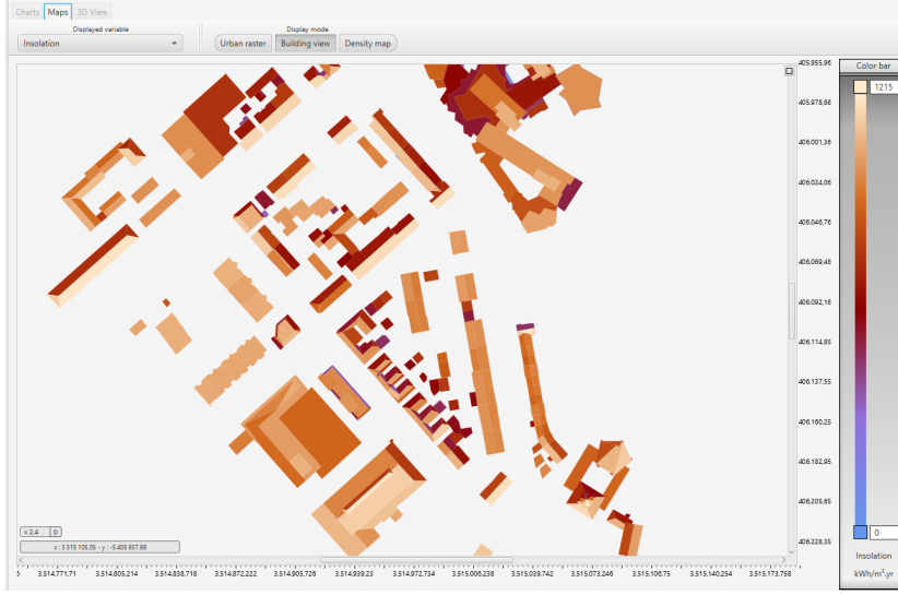
Figure 6.7: Yearly solar irradiance on roofs [kWh/m 2 ].
