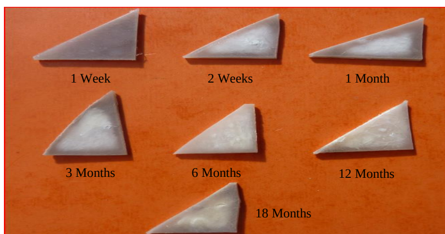
Figure 4-21 (b) Photographs of PCL/10Fe after storage in pH7 solution for up to 78 weeks at 37°C
