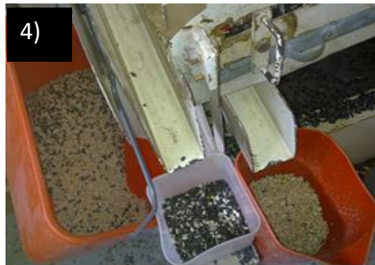
Figure 4:7: De-hulling process (step 1-6) of sunflower seeds in Sutton Bonington Campus, University of Nottingham. The whole sunflower seed (oil seed type) was crushed in a Glen Creston mill then followed by screening to separate the seed coat.
