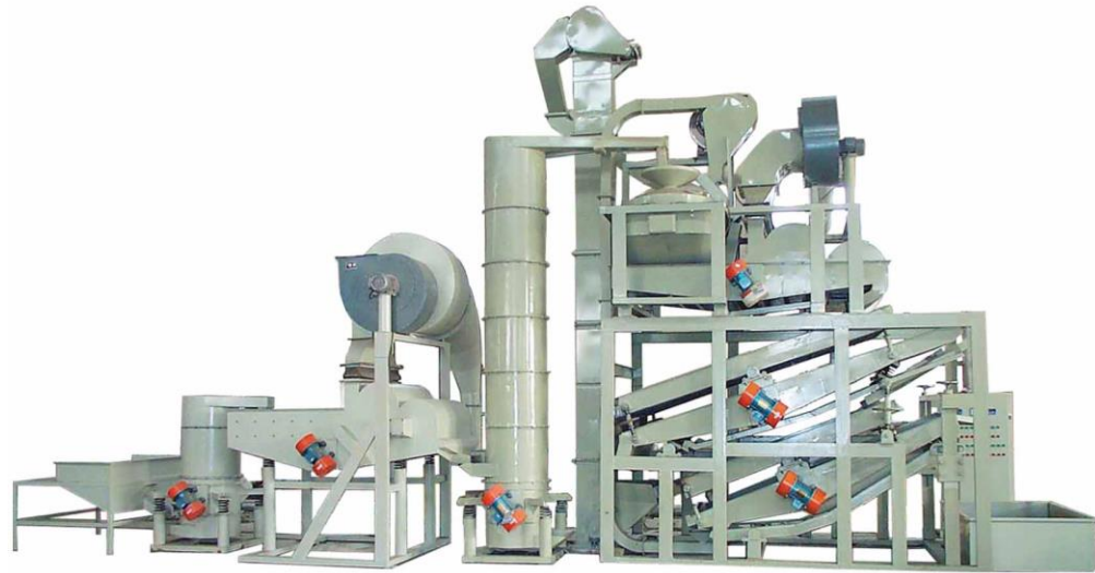
Figure 2:2 Industrial scale of de-hulling machine to separate the sunflower hull with kernel. Source http://www.asia.ru/en/ProductInfo/421697.html
