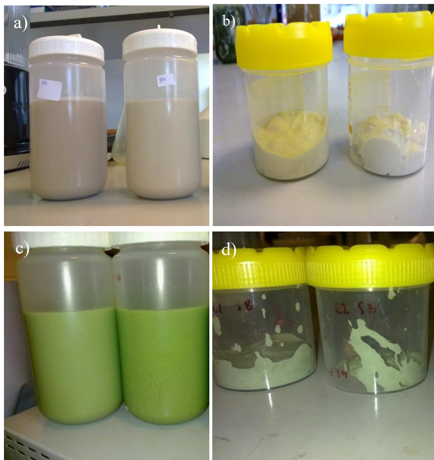
Figure 5:3: Photo showing (a) oil body's milk, (b) oil body's cream, (c) oil body's milk (alkaline grinding medium) (d) oil body cream (alkaline grinding medium). Sunflower seeds were ground with sodium bicarbonate, filtrated and centrifuged before the buoyant cream was obtained. The milk and cream turns to the distinctive green colour due to oxidation when sunflower seeds react with alkaline solution which was used as the grinding medium.
