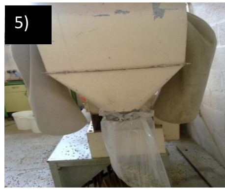
Figure 4:7: De-hulling process (step 1-6) of sunflower seeds in Sutton Bonington Campus, University of Nottingham. The whole sunflower seed (oil seed type) was crushed in a Glen Creston mill then followed by screening to separate the seed coat.
