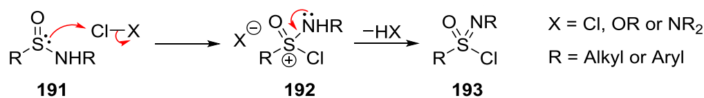
Scheme 1.52. Generalised mechanism for oxidative chlorination.
