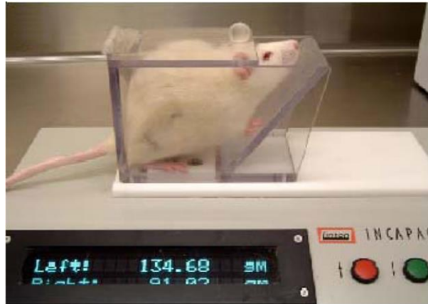
Figure 2.6. Incapacitance meter for the measurement of weight bearing asymmetry. Rats are positioned in a Perspex box placed on the Incapacitance Meter, with each paw lying on a separate transducer pad. The weight borne on each paw for a period of three seconds is recorded. Picture from (Gregersen et al., 2013).
