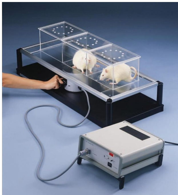
Figure 2.3. Plantar test (Hargreaves method). Rats are placed in Perspex boxes and the source of infrared heat is positioned under the plantar surface of the hindpaw. The controller automatically records hindpaw withdrawal latency. Picture from (BIHEC, 2005-2018).
