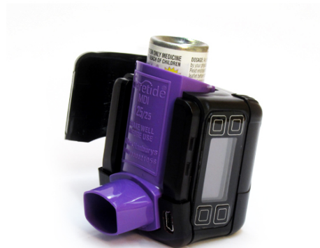
Figure 3-1 – A SmartTrack device (black) clipped around an inhaler (purple)
