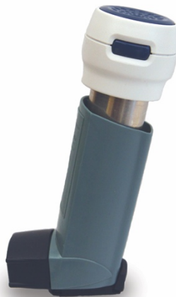
Figure 5-1 - The Propeller sensor attached on top of the canister of an MDI
