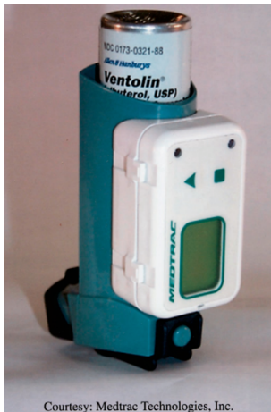
Figure 2-4 – An MDI Log device (white) attached to the back of an MDI
