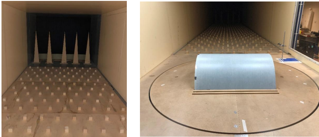
Figure 3-25: a) Spires and roughness elements b) Roughness elements and the structural model placed on the turntable
