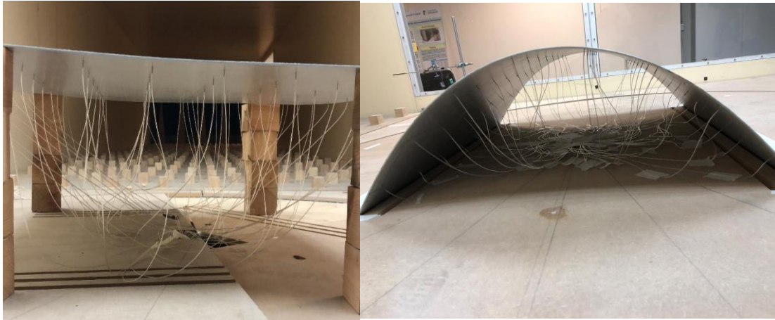
Figure 3-38: installed pressure taps
