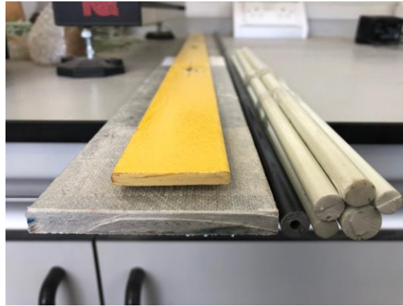
Figure 3-1: Glass Fibre Reinforced Polymer (GFRP) samples
