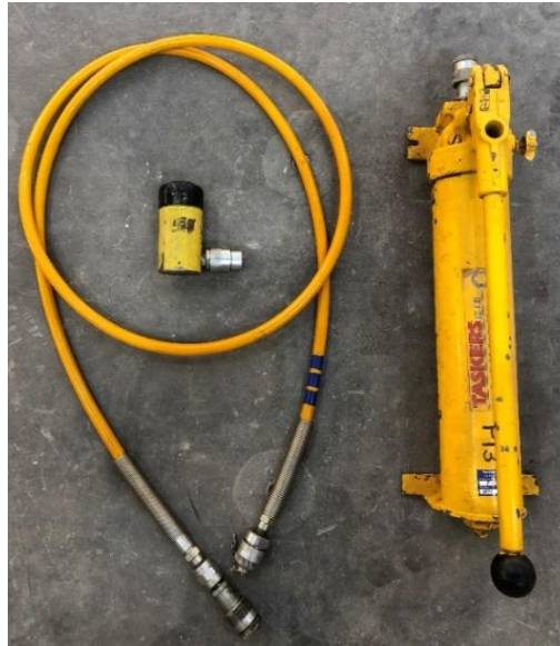
Figure 3-7: Hydraulic Hand Pump with Single Acting Hollow Ram Cylinder
