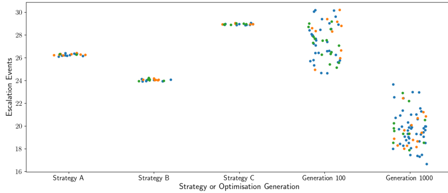
Figure 7.13: Comparison of example AM strategies with optimisation generations for the number of escalation events objective. ● Front 1, ● Front 2, ● Front 3.
